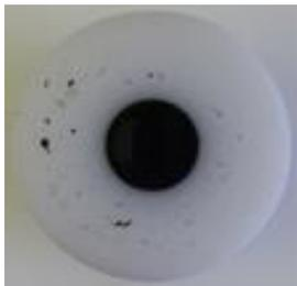
Catalyst detachment after durability test
